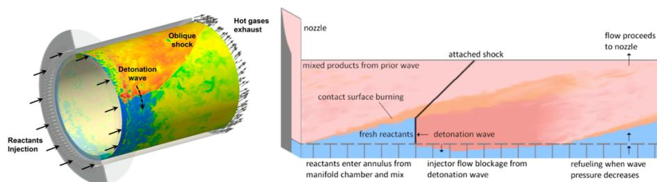
Figure 1. Sketch of typical RDC flow field (Lu, F.K. *et al.*, Journal of Propulsion and Power (2014)).
